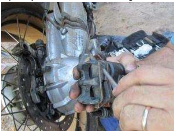
I slowly got round to cleaning up and repairing the brake calliper unit.
